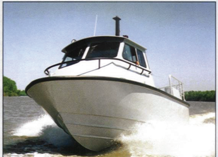
All Dauntless Models Feature Wide Chines, Lifting Strakes And Flared Bows
